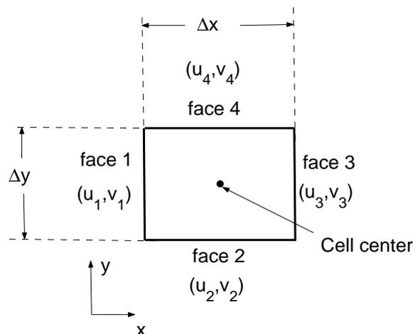
The velocity at face  $i$  is taken to be  $\vec{V}_i = u_i \hat{i} + v_i \hat{j}$ . Applying the mass conservation equation (5) to the control volume defined by the cell gives
