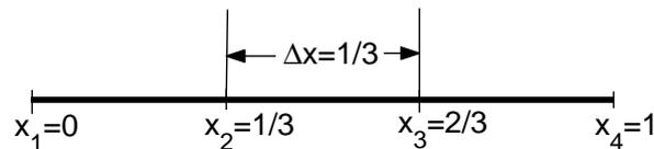
This grid has four equally-spaced grid points with  $\Delta x$  being the spacing between successive points. Since the governing equation is valid at any grid point, we have
