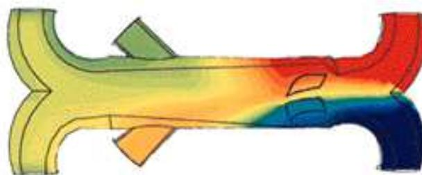
Bio-medical engineering is a rapidly growing field and uses CFD to study the circulatory and respiratory systems. The following figure shows pressure contours and a cutaway view that reveals velocity vectors in a blood pump that assumes the role of heart in open-heart surgery.
