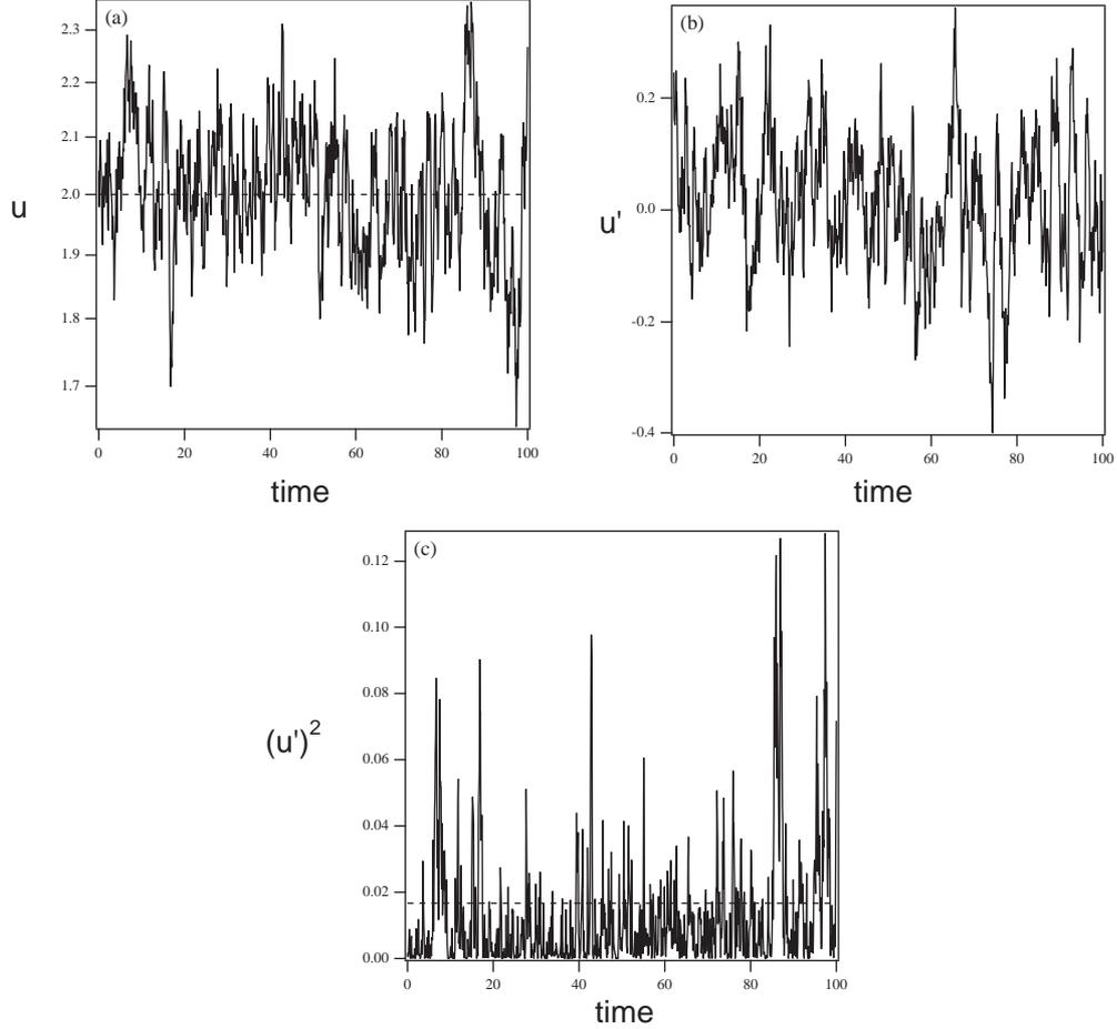
Figure 1: Example of a time history of a component of a fluctuating velocity at a point in a turbulent flow. (a) Shows the velocity, (b) shows the fluctuating component of velocity  $u' \equiv u - \bar{u}$  and (c) shows the square of the fluctuating velocity. Dashed lines in (a) and (c) indicate the time averages.
