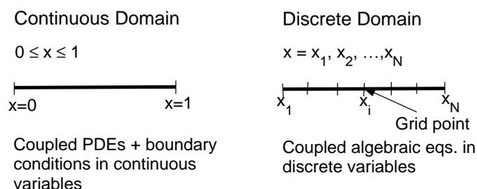
In a CFD solution, one would directly solve for the relevant flow variables only at the grid points. The values at other locations are determined by interpolating the values at the grid points.
