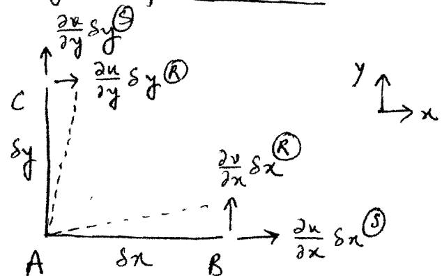
We can observe that the fluid lines will stretch due to the components marked as  $\textcircled{S}$  and rotate due to the components marked as  $\textcircled{R}$ .
