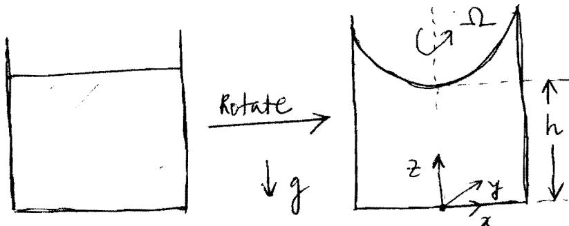
An ideal fluid is rotating under gravity  $g$  with constant angular velocity  $\Omega$ .
