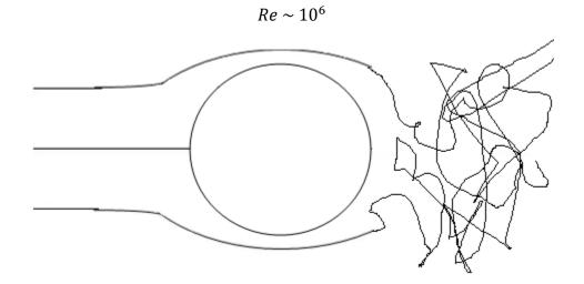
Lack of symmetry in wake suggests lift force in addition to drag force.
