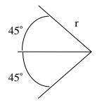
The total distance one wing traverses in a flutter (up and down) motion is  $\pi \cdot r$  or:
