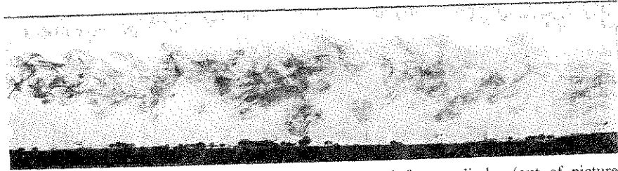
FIG. 3.11 Turbulent wake exhibited by dye emitted from cylinder (out of picture to right). From Ref. [186].
